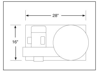
Figure 4. Dust collector footprint.
